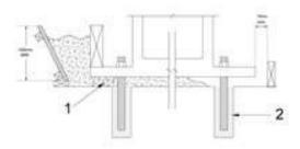
The compressive strength of the grout must exceed 45 N/mm<sup>2</sup> at 7 days and 60 N/mm<sup>2</sup> at 28 days.
