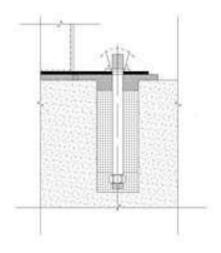
Pouring should be from one side of the void to eliminate any air or presoaked water becoming trapped under the base plate. It is advisable to pour the grout across the shortest distance of travel. The grout head must be maintained at all times so that a continuous grout front is achieved.
